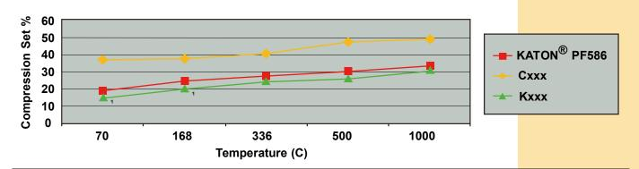
Tests carried out according to ASTM D1414, 25% compression for 70 hours
