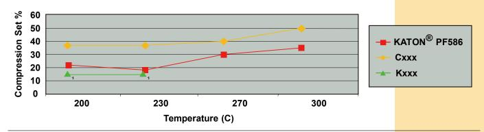
Tests carried out according to ASTM D1414, 25% compression for 70 hours
